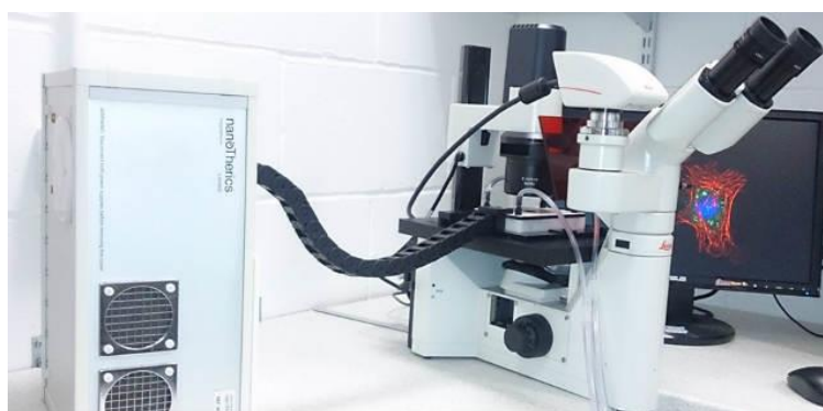
Figure 1: Live Cell AMF exposure system for in vitro time lapse imaging mounted onto a Leica inverted fluorescence microscope.
