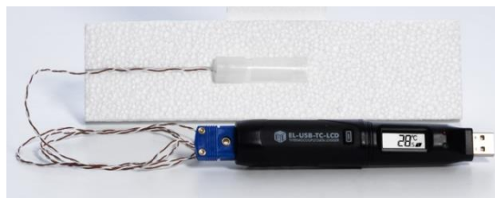
Figure 1. Type T thermocouple and electronics (USB Connection Thermometer)
