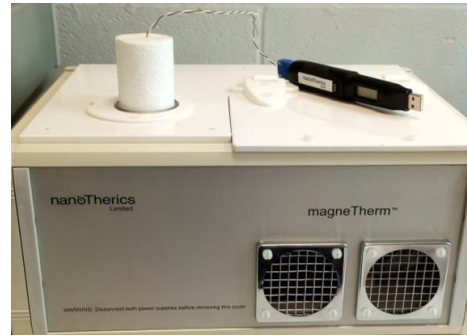
Figure 3. magneTherm's set up with insulating jacket
