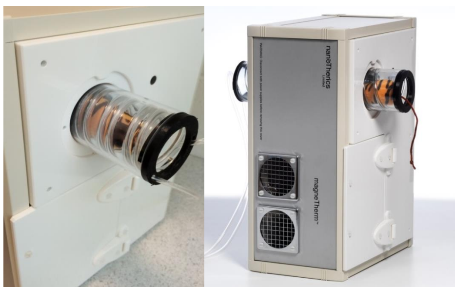
Figure 6. magneTherm's water jacket set up for in vivo / in vitro experiments
