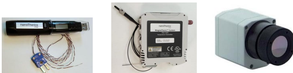
Figure 5. Temperature sensing/ imaging systems compatible with magneTherm i.e. thermocouple with USB Digital Thermometer, fibre optical sensor, infra-red camera
