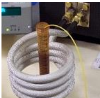
Figure 1. A non-ideal commercial induction heater
