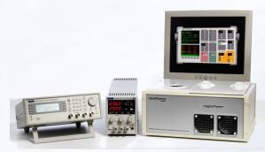
This system includes dedicated software, allowing PC or Mac Control for automated resonance tuning, real time data display and graphing, control of fields strength and exposure times with an option for dual or single channel optical sensors for real time temperature sensing.
