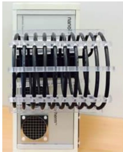
Figure 1: B - magneTherm in vivo external coil setup for rat and rabbit.
