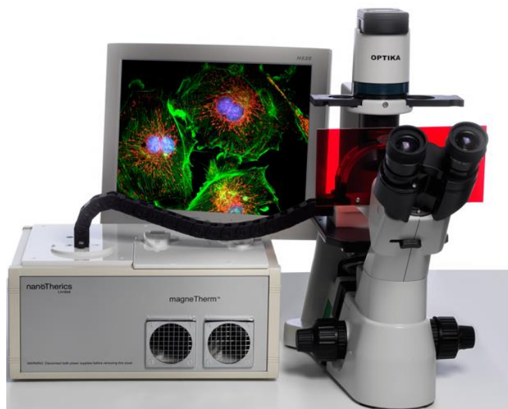
Figure 3: This LC-AMF system can be mounted onto different types of microscopes allowing the microbiologists to understand the mechanisms behind the AMF mediated biofilm treatment real time.
