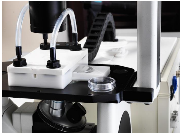
Figure 2: magneTherm provides the option to do experiments in a Petri dish, located within a micro incubator to provide the correct incubation temperature for the microorganisms.
