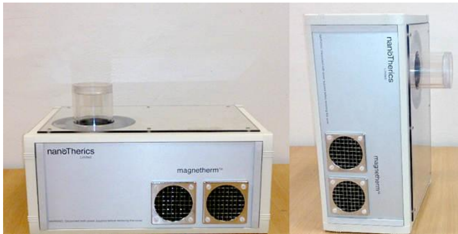
Figure 2: Vacuum chamber to eliminate non-specific heating for calorimetric set up
